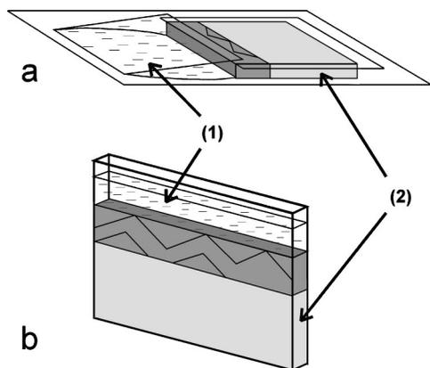
FIG. 1. Experimental setup. The outer electrolyte is denoted by (1), while the inner electrolyte by (2). (a) The gel sheet containing the inner electrolyte is located between a microscope slide and a cover glass. The outer electrolyte is dropped to an edge of the gel sheet, and protected by another cover glass. (b) The gel sheet is located between two glass plates. The outer electrolyte is layered on the gel.
