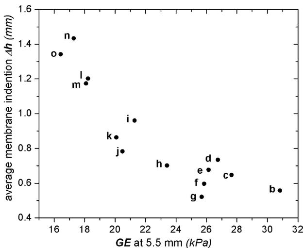
Fig. 6. Averaged membrane indentation values ( $\overline{\Delta h}$ ) when the outstanding region was pressed by a force of 1.3 N, vs. the generalized elastic modulus GE measured at 5.5 mm deformation of the samples. Note the correlation between  $\overline{\Delta h}$  and GE. Again, the point representing sample “a” ( $\overline{\Delta h} = 0.22$  mm, GE = 163.68 kPa) is not figured.
