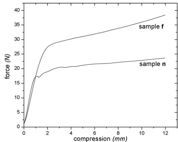
Fig. 4. Compression–force diagram of samples “f” and “n”.
