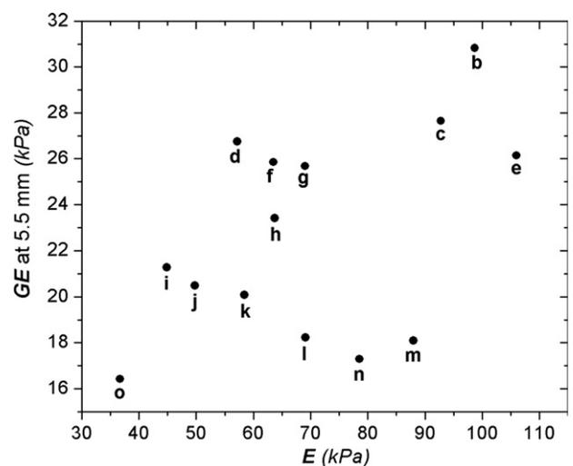
Fig. 5. General compression elastic moduli (GE) measured at 5.5 mm vs. compression–Young moduli ( $E$ ) of the investigated sponge samples. There is no correlation between these elastic parameters. The point representing sample “a” ( $E = 222.74 \text{ kPa}$ ,  $GE = 163.68 \text{ kPa}$ ) is out of the range of the figure.
