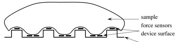
Fig. 2. Schedule of a device for measuring the elastic parameters, with force sensors in its outstanding and indenting regions. The device is pressed to the investigated sample, that folds into the indenting regions. Signals of the force sensors enable the calculation of the elastic moduli of the sample.
