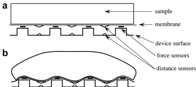
Fig. 1. Schedule of a device for measuring elastic parameters, having force and distance alternation sensors. When the device just touches the investigated sample, the sensors do not show signals (a). If the device is pressed to the specimen, the signals of the force and that of the distance alternation sensors enable the calculation of the generalized elastic moduli of the sample (b).
